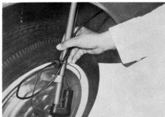
Fig.4-12 Antenna Removal V0973
